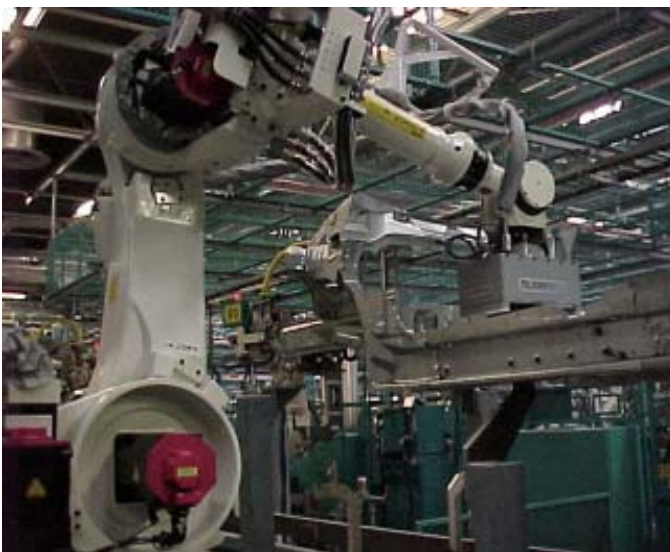
A robot positions the TeleScribe® within the on-line marking station at NedCar BV.
