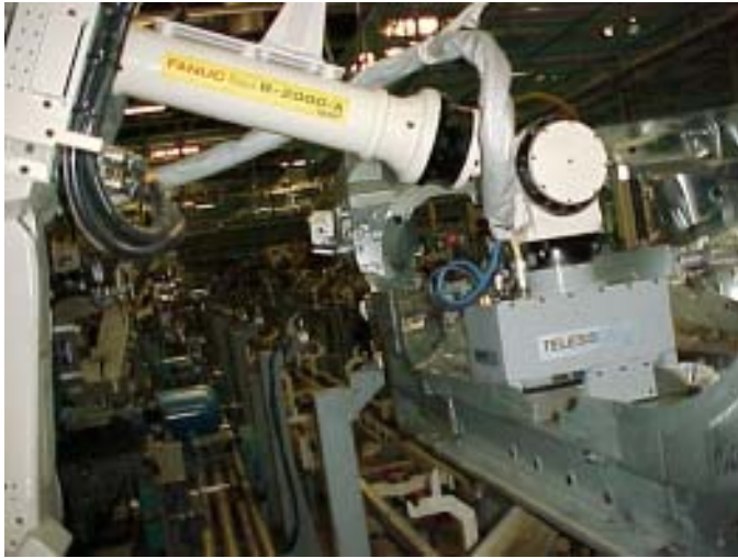
Completely automated Marking Process.
