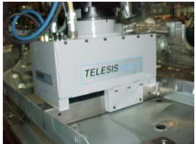
Telesis Servo-Driven TeleScribe® Marker clamped onto the body panel.
